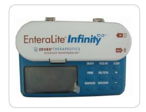
2 Press the RATE/DOSE key to display the rate (see the bottom left corner of the screen). Program the prescribed rate using the (+) and (-) keys.
