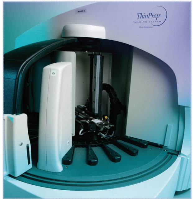
Shown above is the Thinprep Imager, capable of imaging 400 slides per 24-hour period. Intermountain has two Imagers.
