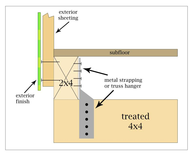
Take note that the exterior sheeting is NOT flush with the 2x4. When the forklift slides beween the 4x4s and picks up the playhouse by the 2x4s, the drag of the forks as they back away pull the sheeting and exterior from the framing if flush.
