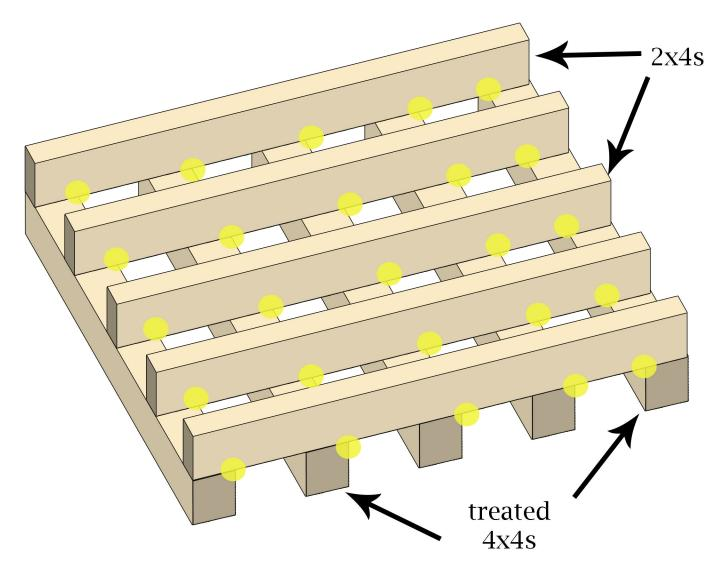
Use a metal truss hanger or strap at each intersecting point to securly attach the 2x4s to the 4x4s.
