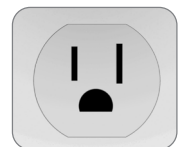
A grounded outlet has 3 holes
